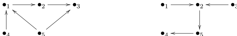
Figure 1.5.4: Left: \{1, 4\} and \{3\} are d -separated by \{2, 5\} , but not by \emptyset , \{2\} or \{5\} . Right: \{1\} and \{3\} are d -separated by \emptyset , but not by any nonempty subset of \{2, 4, 5\} .
